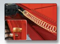
✓ Convenient air source for tools at front and rear
