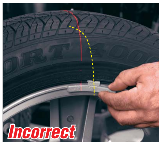
Angle errors from even slight misjudgment of the TDC location lead to an inferior and time-consuming balance with excessive checkspins.
