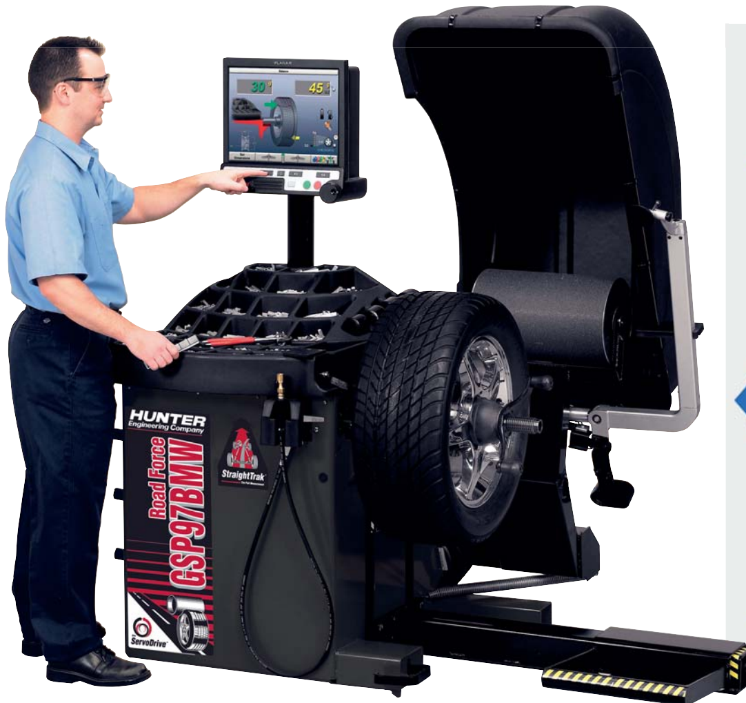
Shown with optional Wheel Lift system and optional StraightTrak LFM feature.
