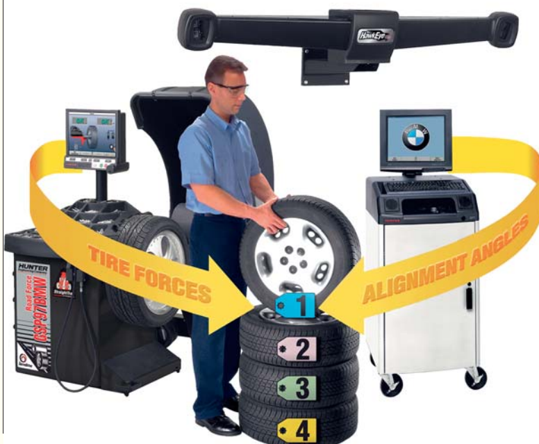
Tires are tagged and positioned on the vehicle to provide the least amount of vehicle pull and obtain the best straight ahead
