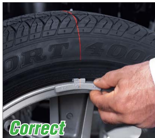
Precision wheel weight placement is fast and easy using the HammerHead TDC laser as a guide.
