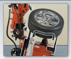
Eliminates manual lifting. Polymer-coated wheel-contacts protect the finish on custom wheels. (20-2201-1)
