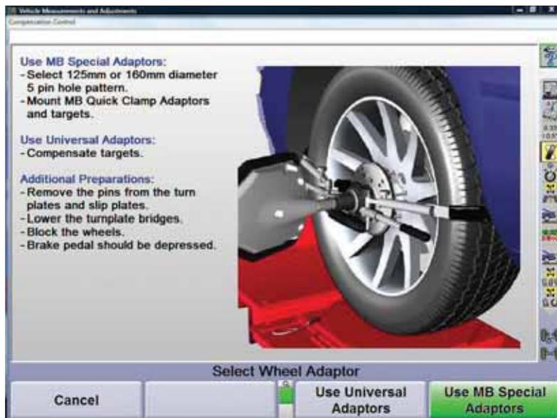
**The Mercedes-Benz customized WinAlign alignment software provides easy-to-follow vehicle-specific procedures to simplify alignment service.**
