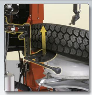
**Demounting with locking arm**Demount heavy tires and stiff bottom beads with roller. Saves having to lift heavy tires!
