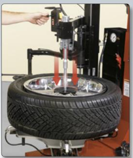
Pneumatic wheel press cones and extension arm simplify external alloy wheel clamping when servicing low-profile tires.
