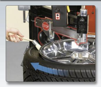
Tapered rollers assist in bead lubrication and bead lever placement to ease demounting.
