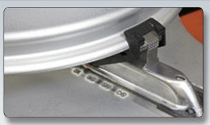
**External clamping for alloy wheels**Measurement marks aid external clamping.
