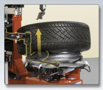
The bottom roller disc assists in reloosening tire beads and lifting the tire up the wheel barrel during demounting.
