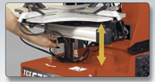
Two work positions help service narrow and wide wheels and adjust to tall or short operators.
