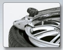
Drop-center clamp (RP11-8-11400070) can be used as a traction point or bead guide. Guides bead into drop-center.
