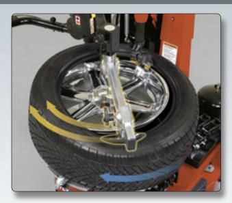
A single bead press roller with rotating arm can quickly be used for mounting and demounting stiff sidewall tires.
