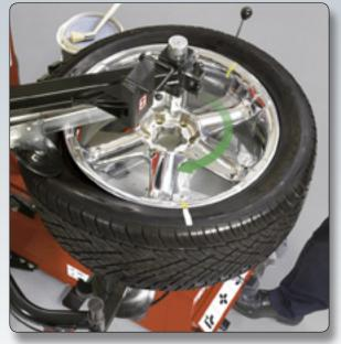
**Match-mounting made easy with the TCX575**Lower locking arm allows operator to spin the tire on the wheel regardless of aspect ratio or tire stiffness.
