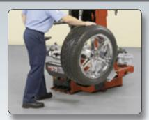
Optional wheel lift (20-2044-1) eases servicing of large assemblies. Allows for more careful handling of expensive wheels.
