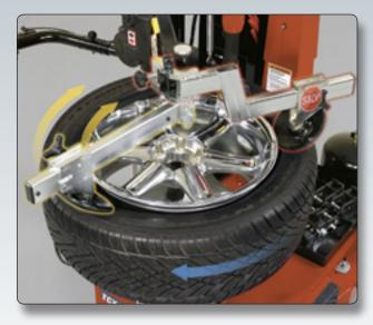
When combined with the rotating arm, the fixed bead press arm adds additional bead pressing force to service the most extreme low-profile tires and deep drop-center alloy wheels.
