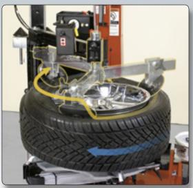
Rising cam rollers expertly guide the bead through mounting.
