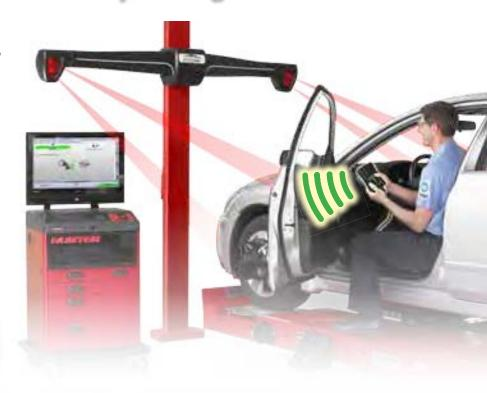
Steering system reset typically involves resetting the steering angle sensor, but on some vehicles, torque angle, yaw rate and other steering-related sensors are also reset.
