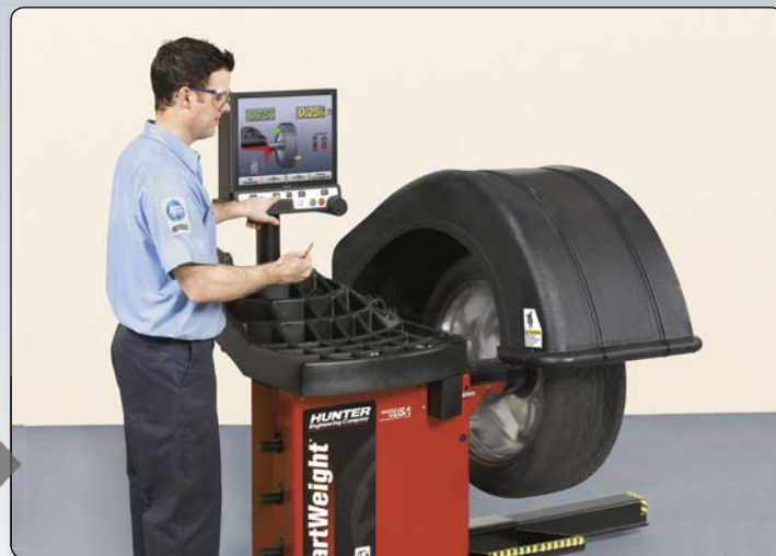
Technician prepares correction weights
