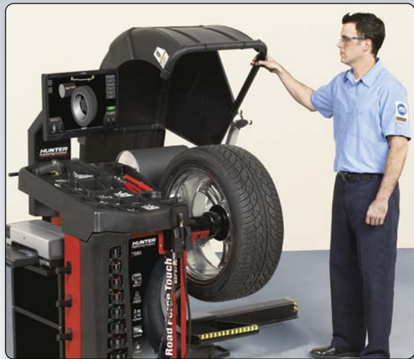
Road Force Touch® balance starts when hood is lowered
