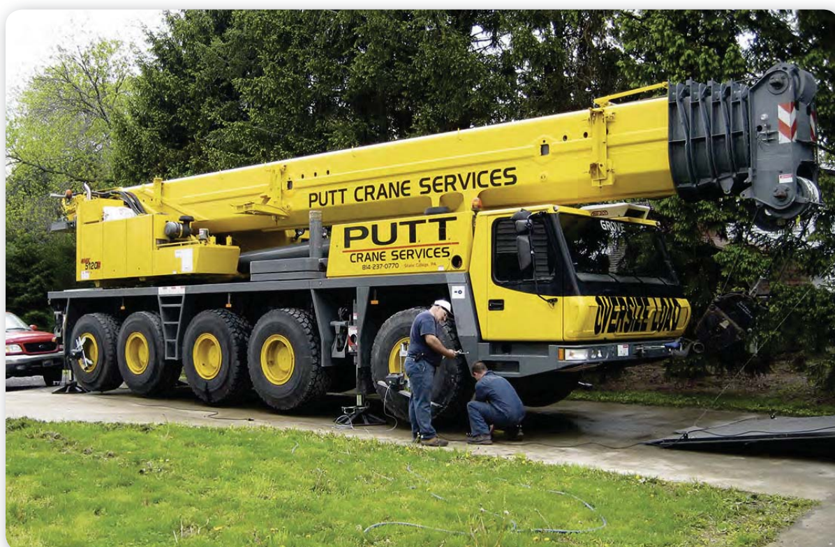
Hunter HD Equipment Specialist Dennis Steffler, with the assistance of a local Purcell Tire alignment technician, align the 60-ton, five-axle crane.
